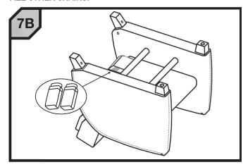
Tilt chair upside down and locate battery backup door on side of control box (it has a silver label on it). Remove the door and install two 9V batteries.
