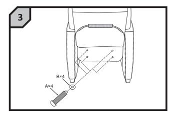
Insert and tighten all bolts as shown. Use allen wrench to fully tighten.
