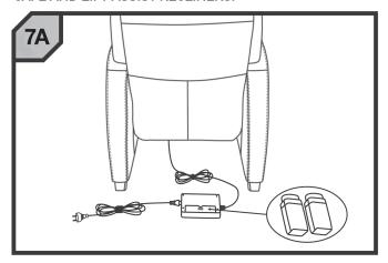
Insert two 9V batteries into compartment shown for backup power.
